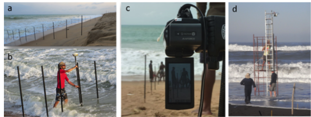
In-situ deployment of metrological techniques. a) extraction of cross-shore profil using a measurement stick, b) GPS localisation, c) HD camera and d) LIDAR.
