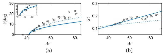
FIG. 2 (color online). Bifurcation diagram for a spiraling disk with  $\chi = 6$  and  $\bar{\rho} = 0.99$ : (a) inclination angle; (b) frequency. Same convention as in Fig. 1, i.e., the solid (dashed) line now corresponds to the RW (SW) branch.
