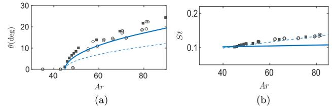
FIG. 1 (color online). Bifurcation diagram for a fluttering disk with  $\chi = 3$  and  $\bar{\rho} = 0.99$ : (a) inclination angle; (b) frequency. The solid (dashed) line corresponds to the stable, i.e., SW (unstable, i.e., RW) branch. The open and closed symbols are data from experiments [26] and DNS [27], respectively.
