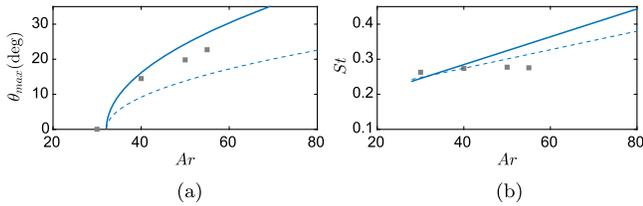
FIG. 3 (color online). Bifurcation diagram for a fluttering oblate spheroidal bubble with  $\chi = 2.5$  and  $\bar{\rho} = 10^{-3}$ : (a) inclination angle; (b) frequency. Same convention as in Fig. 1. The square symbols are DNS data from Ref. [11].
