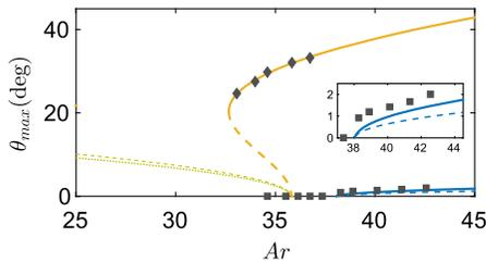
FIG. 4 (color online). Bifurcation diagram of the inclination angle of an infinitely thin disk with  $I^* = 4 \times 10^{-3}$ . Same convention as in Fig. 1 for the solid and dashed lines, the left (right) pair of which corresponds to the subcritical (supercritical) bifurcation. The two series of closed symbols are DNS data from Ref. [28]. The S-shaped curve is an empirical fit based on an extension of Eq. (3) up to terms of  $O(\epsilon^5)$ .
