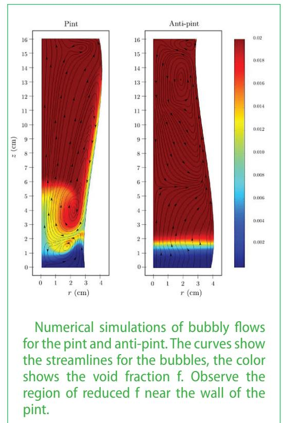
Numerical simulations of bubbly flows for the pint and anti-pint. The curves show the streamlines for the bubbles, the color shows the void fraction  $f$ . Observe the region of reduced  $f$  near the wall of the pint.
