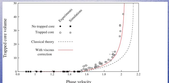
Transport volume versus phase velocity according to our experiments and simulations (symbols), classical theory, and our modified model accounting for viscous effects.
