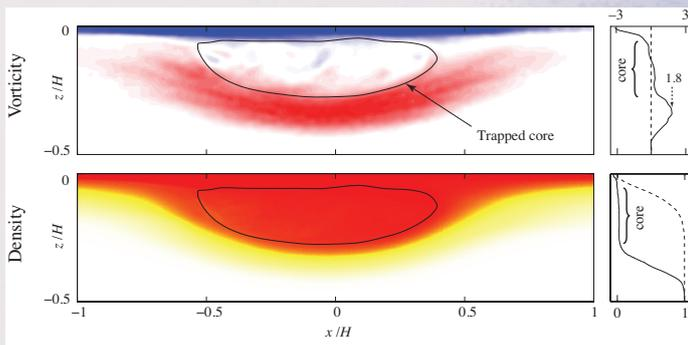
Normalised vorticity (top) and density (bottom) fields for a solitary internal wave with a trapped-core. The black contours denote the core region. The right-hand panels show vertical profiles at the wave trough; dashed lines show background conditions.
