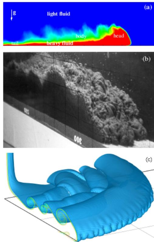
**Fig. 1** Gravity current structure. Frame (a) shows schematically the structure of a gravity current. Frame (b) shows the front of a planar gravity current from a laboratory experiment. Picture courtesy of Marcelo H. García. Frame (c) shows a still of the flow in a circular sector of  $\pi/2$  from the simulation of the cylindrical gravity current. The flow is visualized by a density isosurface.
